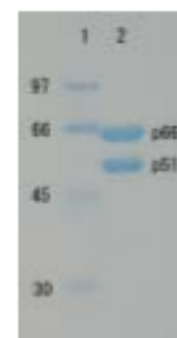
Fig. 1 Polyacrylamide gel electrophoresis of HIV-1 reverse transcriptase protein
